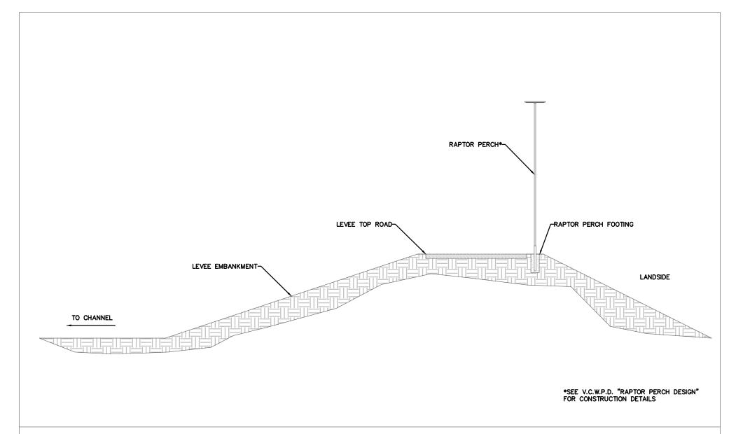
LEVEE CROSS-SECTION PROFILE WITH RAPTOR PERCH
